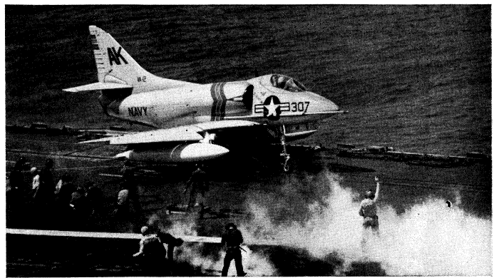
Douglas A4D "Skyhawk" making preparations for take-off from a canted-deck carrier. Flight deck officer (right) guides the pilot with a series of hand signals
