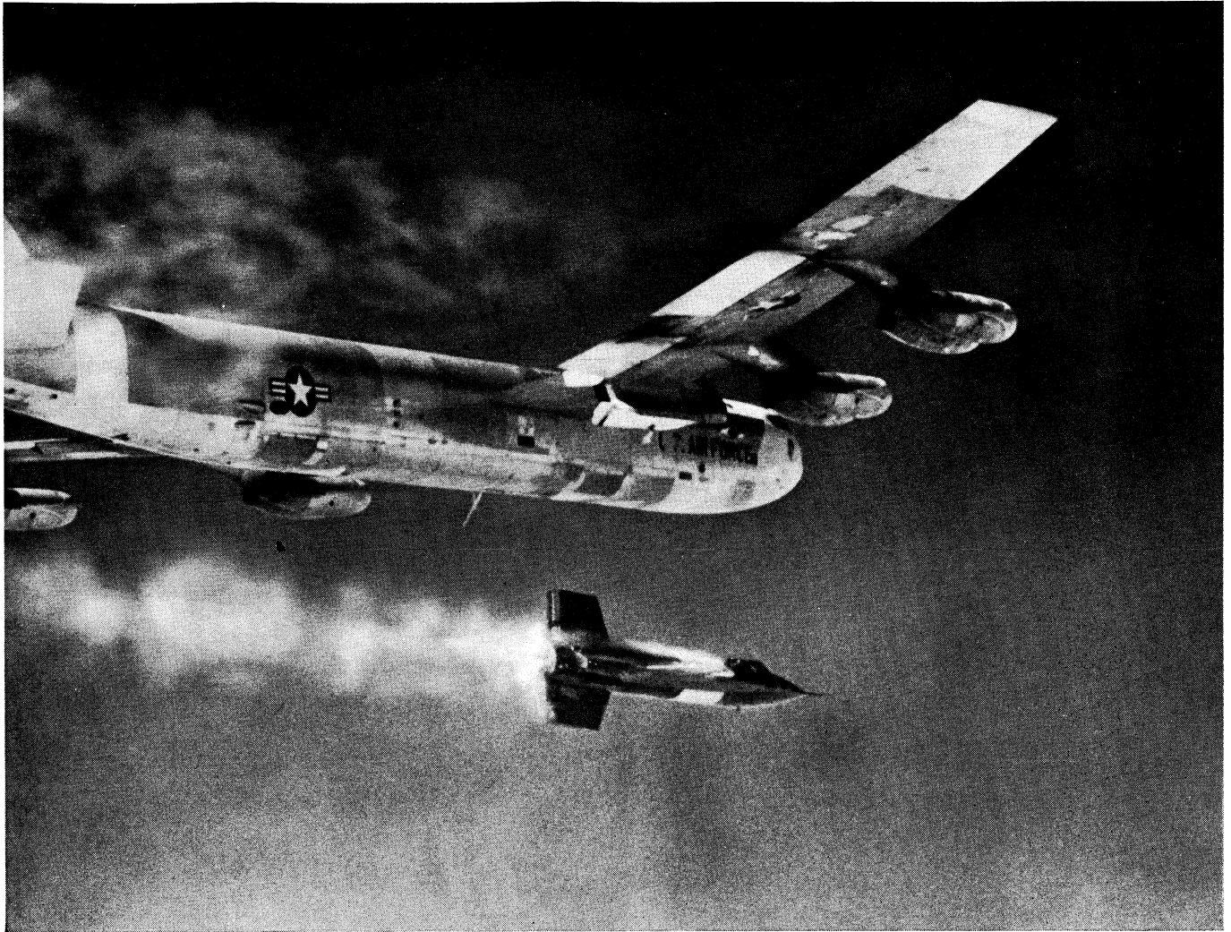
B-52 Stratofortress bomber at 45,000 ft. dropping the X-15 space research rocket plane after pilot has ignited the engine
