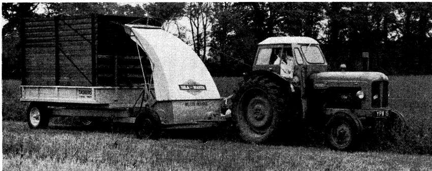
Harvesting a crop of lucerne (alfalfa) on a farm in England with a tractor-mounted forager which cuts and chops for ensilage
