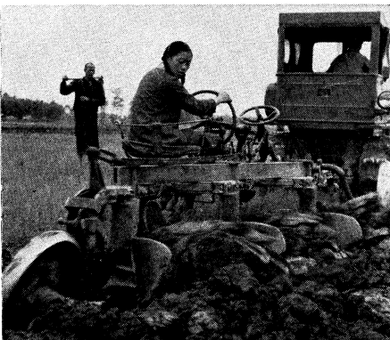
Two-man multi-bladed disk plow being operated at a co-operative farm in China
