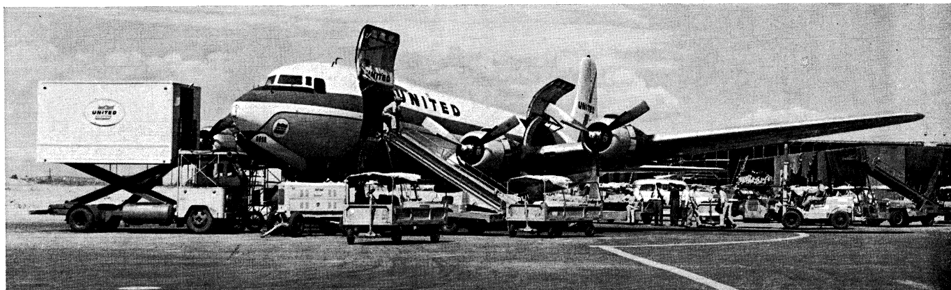
Loading operations at the cargo terminal of Stapleton airfield, Denver, Colo. Freight is being loaded into a Douglas cargo aircraft by means of mobile, power-driven conveyor ramps
