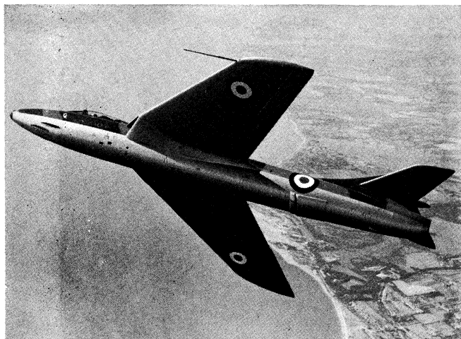
British Hawker Hunter, swept-wing, jet-propelled fighter powered with Rolls Royce Avon or Siddeley Sapphire engines
