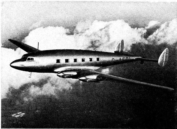
De Havilland Albatross, British four-engine transport of 1937, a low-wing monoplane which seated 20-30 passengers
