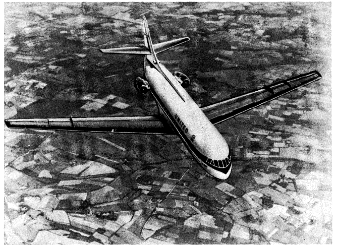
Sud-Aviation Caravelle, French jetliner, 1955. With twin engines by Rolls Royce, Ltd., it carries up to 80 passengers at 480–500 m.p.h. for 1,200 mi.
