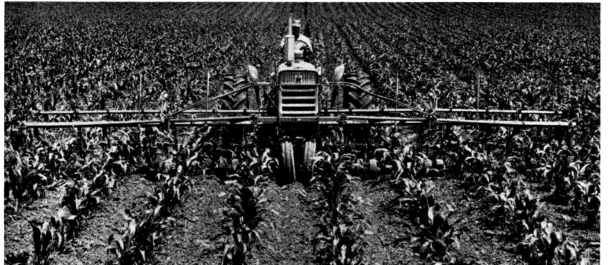
Diesel-powered tractor mounted with an eight-row cultivator being used in a U.S. cornfield
