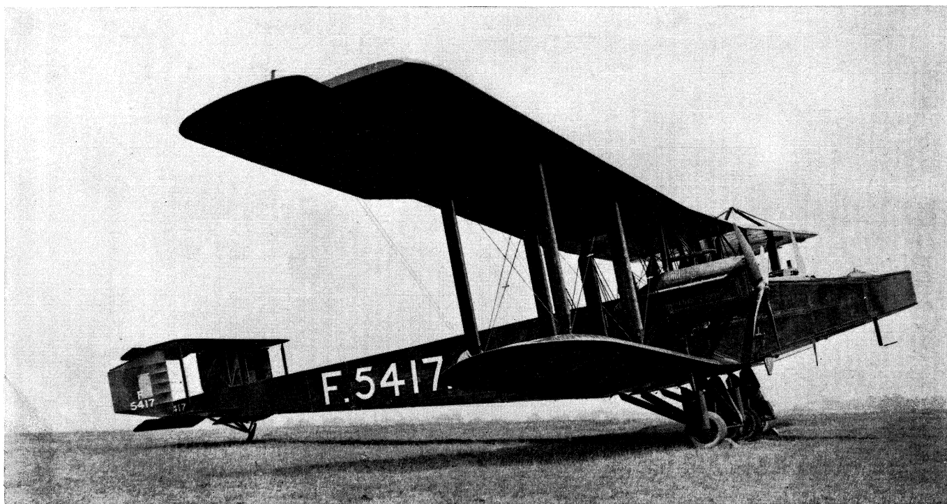
Twin-engined Handley Page 400, 1917. The first British heavy bomber, it flew at 60–80 m.p.h. carrying a bomb load of 1,800 lb.
