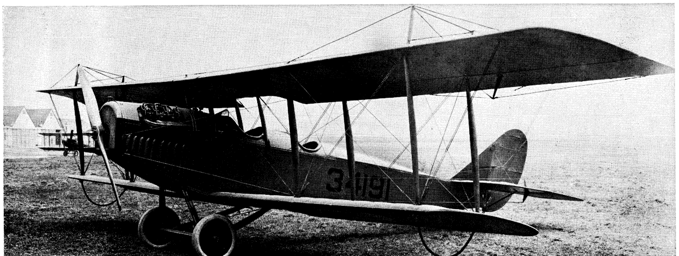
The Curtiss JN-4 "Jenny," one of the series of Curtiss single-engined planes used to train U.S. pilots during World War I
