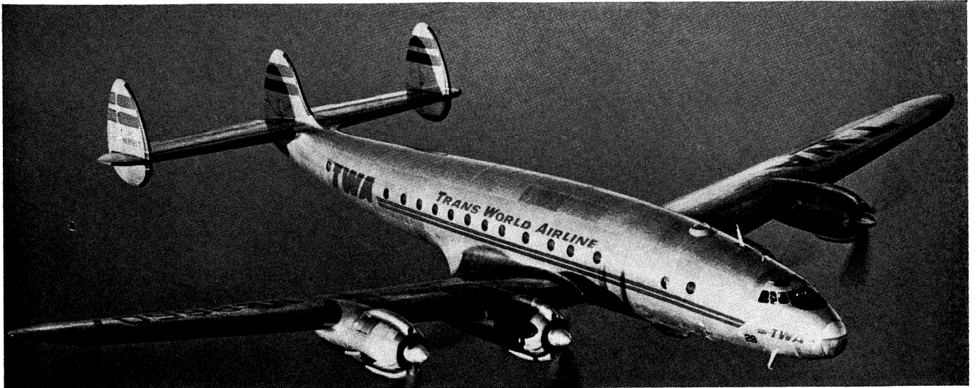
Lockheed Constellation, 1943. This four-engine airliner carries up to 65 passengers at 260–300 m.p.h. for 2,000–3,000 mi.
