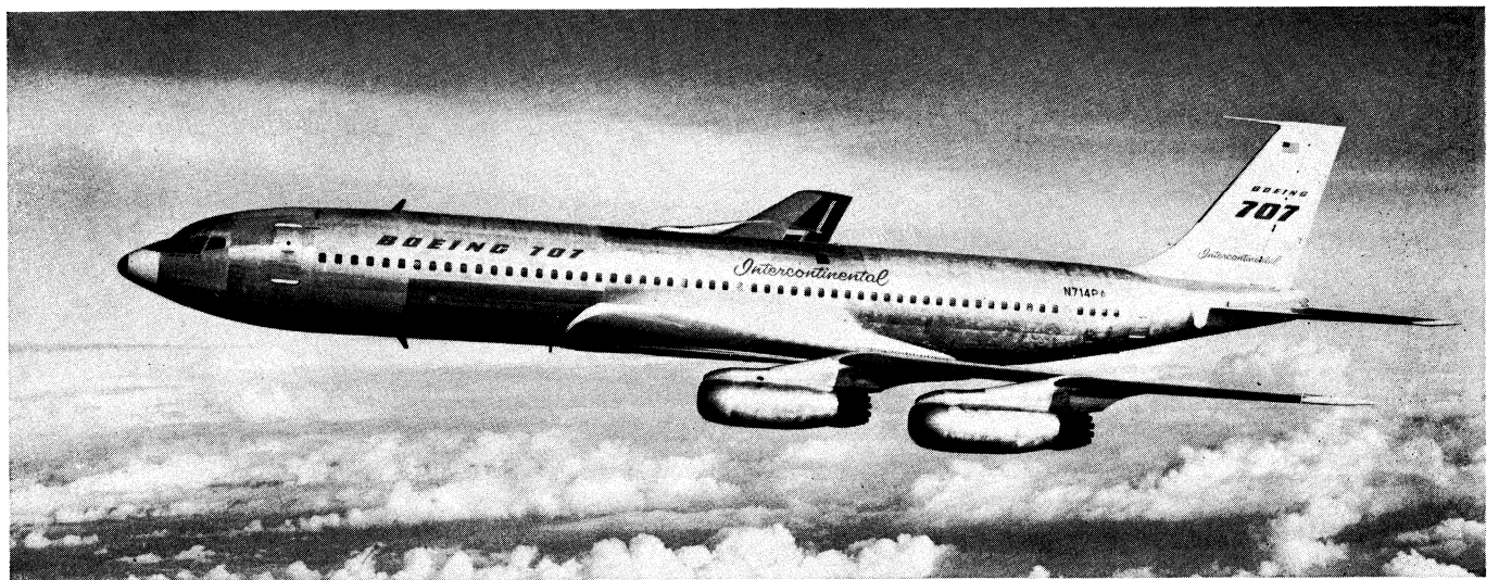
Boeing 707 Intercontinental, 1959. This U.S. jet carries up to 160 passengers at 550 m.p.h. for 3,500 mi.
